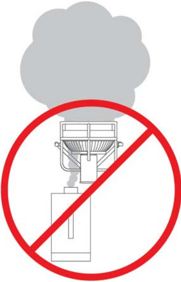
Incorrect ProFan placement in front of fogger/hazer
